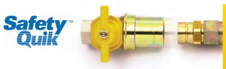
With **Safety Quik** the hose can only be disconnected when the valve is turned to the OFF position. Gas flow is safely shut off with a simple, one-handed action. Likewise, the valve cannot be opened until the gas hose is correctly re-attached. Thermal shut-off safety
